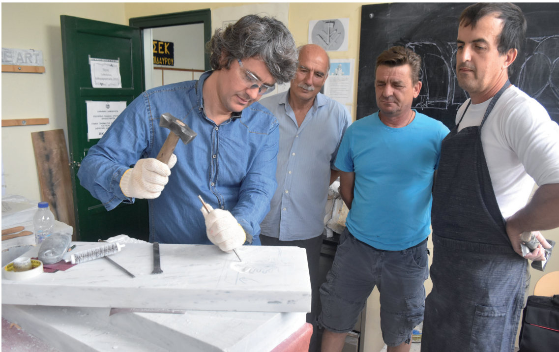
Fig. 6: After finishing the work, he cuts off the slab from the raw part of the marble block.
