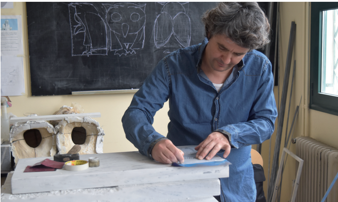
Fig. 2: The first stage after selecting and transferring the appropriate piece of marble is to sketch the motif on its smooth surface.
