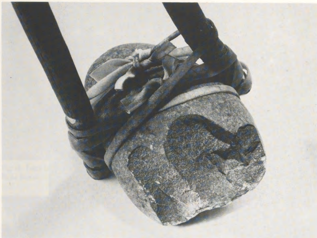
Fig. 15 Mining hammer after several hours use in mining experiments against fireset rock. The notched hammerstone is lashed to the handle with rawhide.
