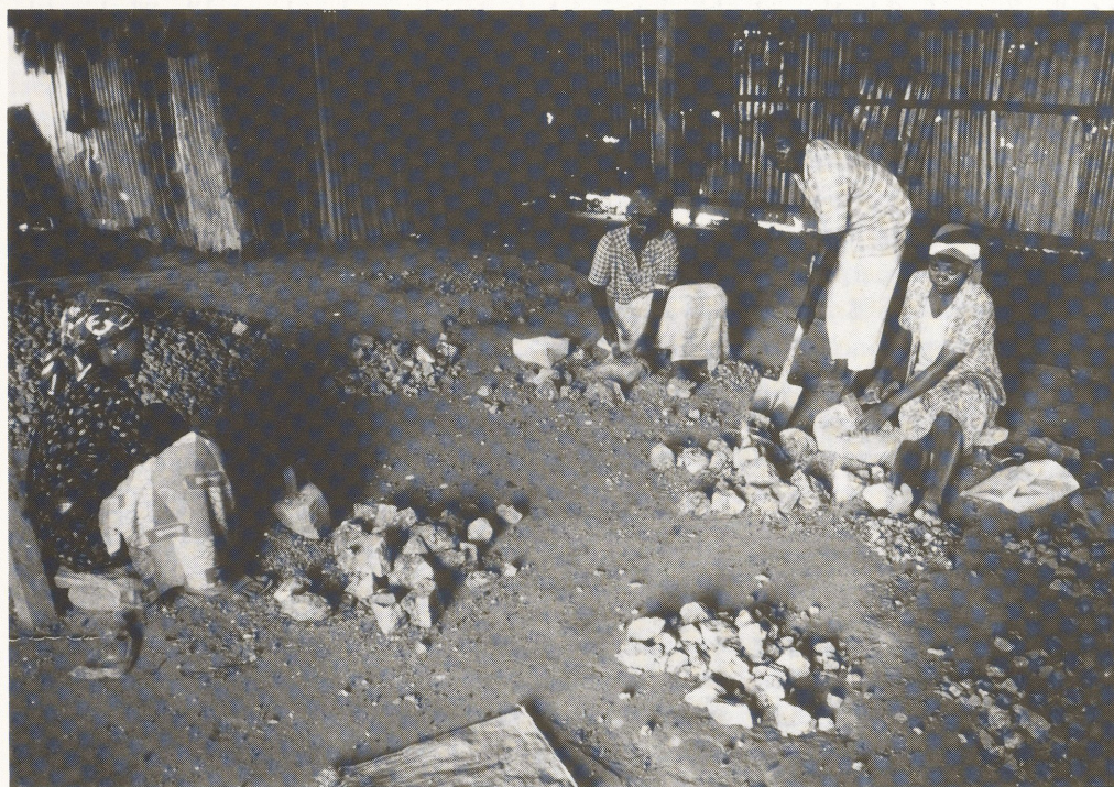
Fig. 19 Crushing and hand-sorting galena and sphalerite at Ishiagu, Nigeria, December 1989.
