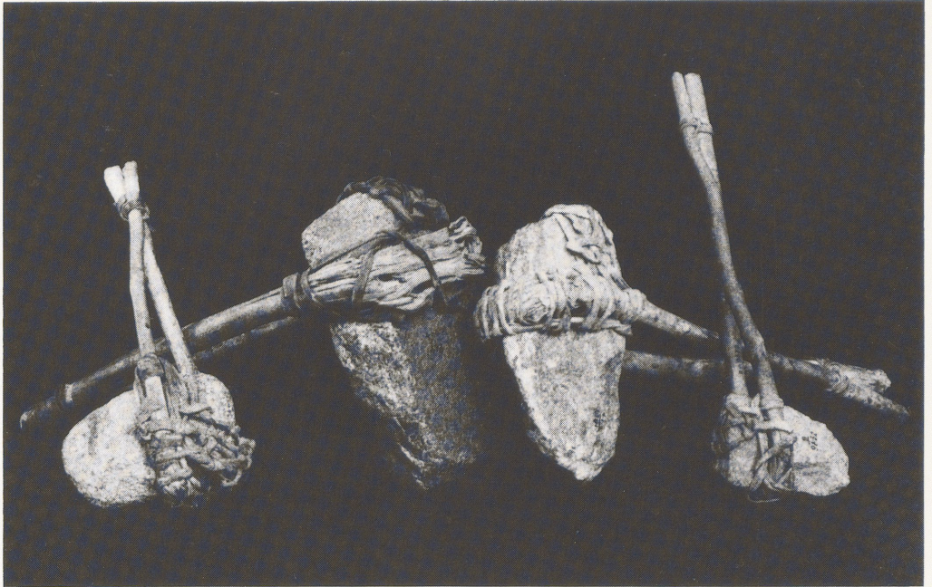
Fig. 14 Selection of stone mining hammers still with their wooden handles, found with the 'copper man' from Chuquicamata, Chile (from BIRD 1979).
