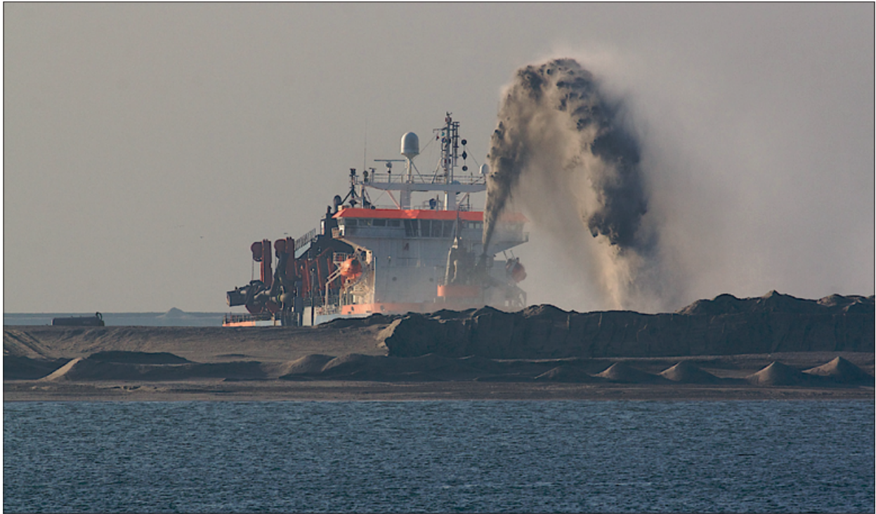
Fig. 7 Trailing suction hopper dredger creating new land (Maasvlakte 2) using Pleistocene sediments, including fossils, from the Eurogeul area. – (Photo H. Wildschut).
