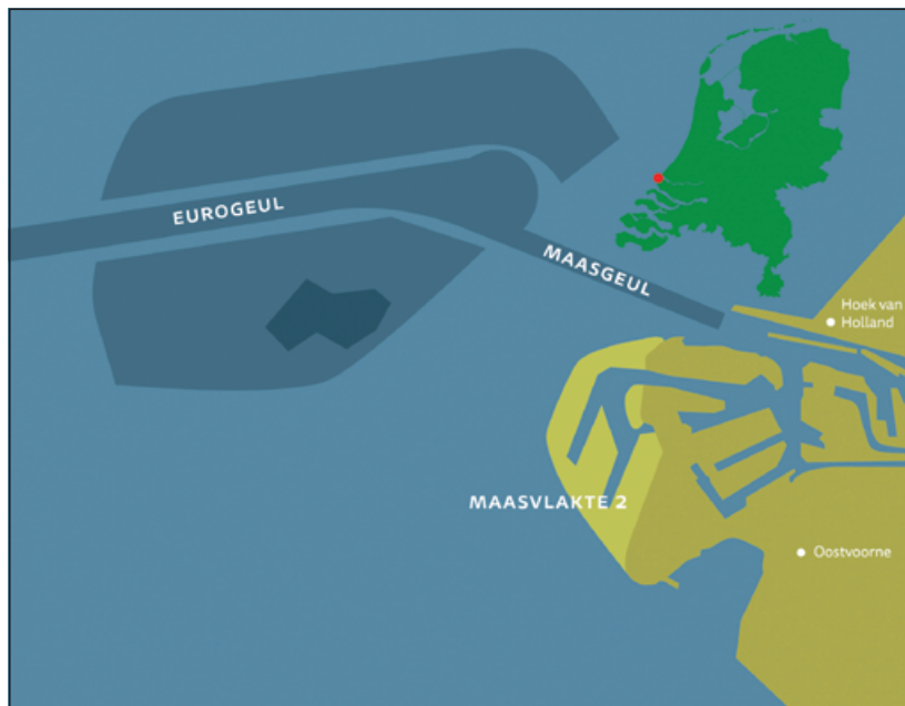
Fig. 6 Schematic view of Maasvlakte 2 and the Eurogeul area, including the sand source area off the coast of the province of Zuid-Holland. Inset: location of Maasvlakte 2 (red dot) in the Netherlands. – (Map J. van Leeuwen / J. Streutker).
