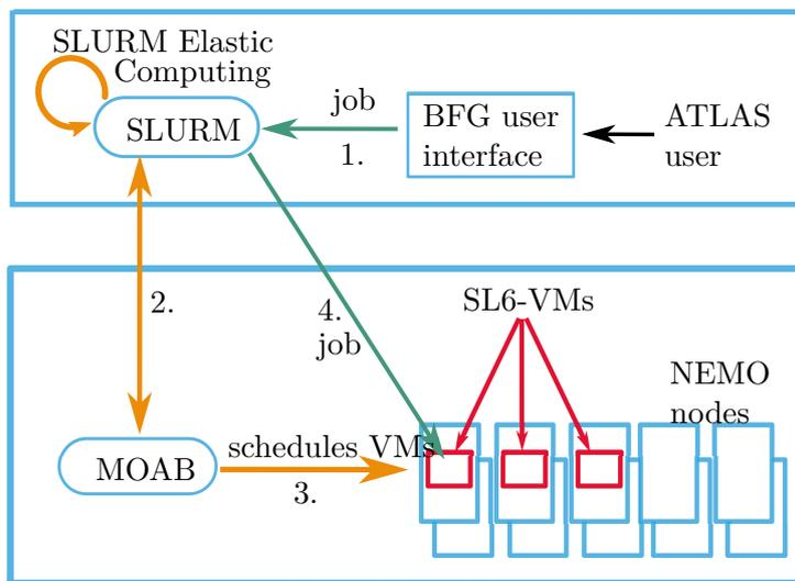
Figure 2: Virtualization environment for ATLAS on NEMO.
