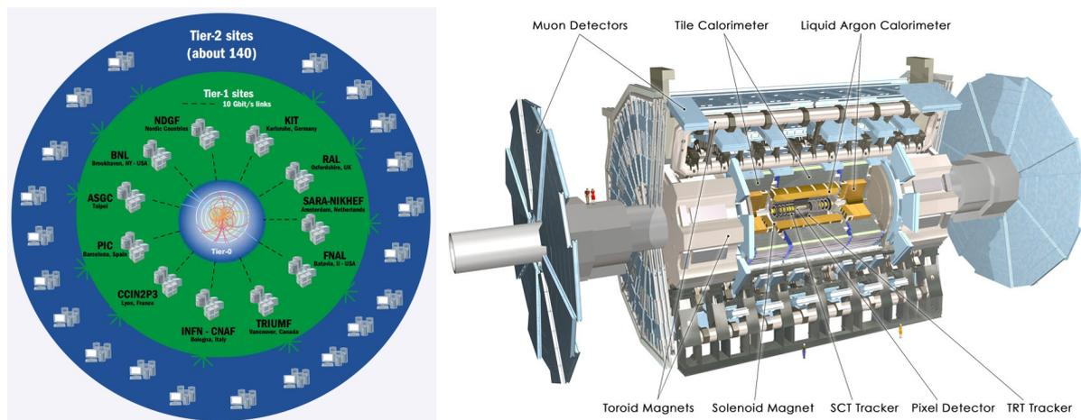
Figure 1: Left: Structure of the WLCG<sup>1</sup>. Right: Schematic of the ATLAS experiment<sup>2</sup>.
