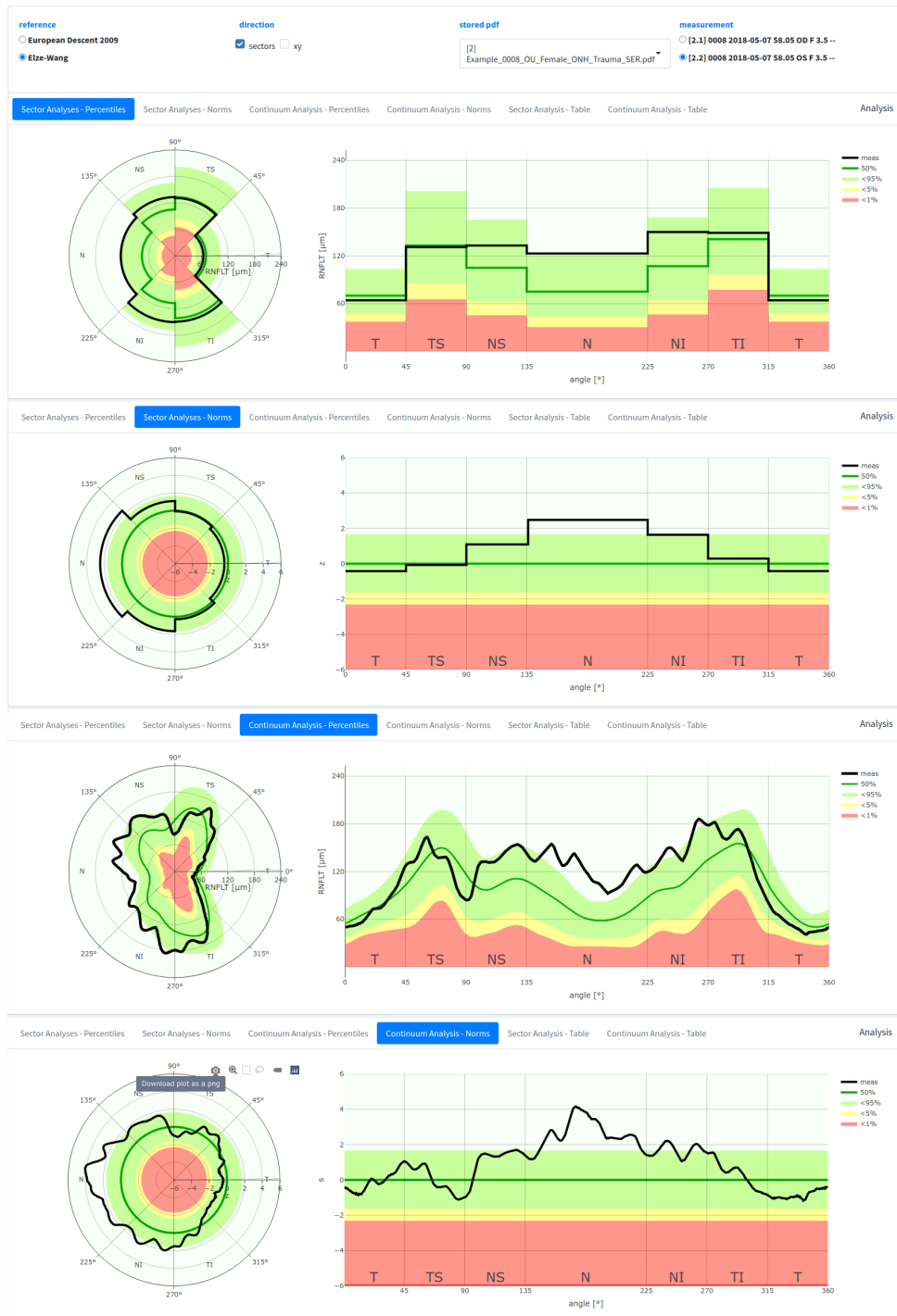
Figure 2: Montage of the 4 provided RNFLT-Visualization. All pictures show the patient's data against percentiles background (1%, 5% and 95%) related to the selected normative data. The sector analyses use norms averaged on the sectors. The continuum analyses use normative data for each of the 768 measure points. The graphs in the pictures 1 and 3 are plotted in real space where the graphs 2 and 4 are plotted in z-space. In the left column we have polar plots and in the right one filled line charts. The visualizations can be selected by tabs on the top. RNFLT is evaluated in six sectors (T: temporal, TS: temporal-superior, TI: temporal-inferior, N: nasal, NS: nasal-superior, NI: nasal-inferior) and overall average (G; used in table only).
