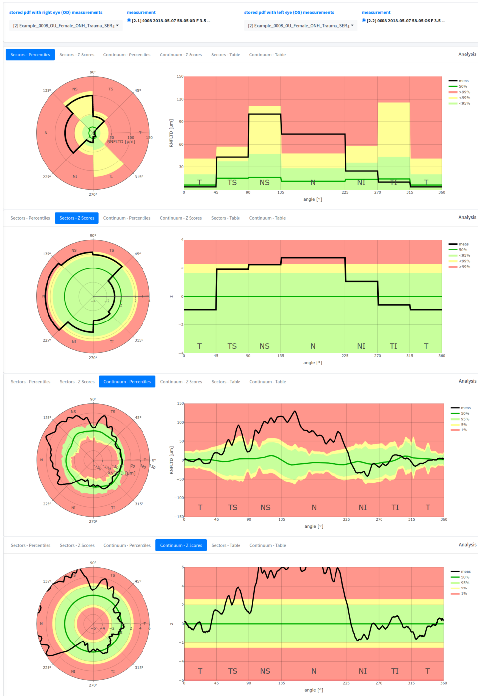
Figure 3: Montage of the four provided RNFLTD presentations. All graphs show the patient's data against percentiles background (1%, 5% and 95%) related to the selected normative data. The sector analyses use Elze-Wang Box-Cox-T normative data computed for each sector. The continuum analysis employs normative data for the difference of each of the 768 measuring points of both eyes. The first and third graphs are plotted in real space whereas the second and fourth graphs are plotted in z-space. Similar to the RNFLT plots, the left column depicts polar plots and the right column depicts filled line charts.
