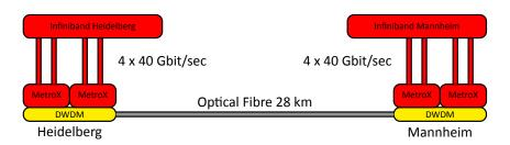
Figure 2: bwForCluster MLS&WISO: Long-distance Infiniband interconnect.
