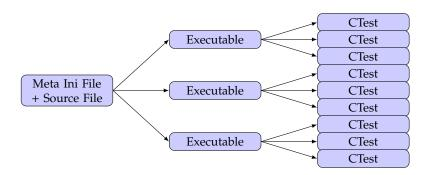
Figure 2: Expansion procedure for the macro dune\_add\_system\_test
