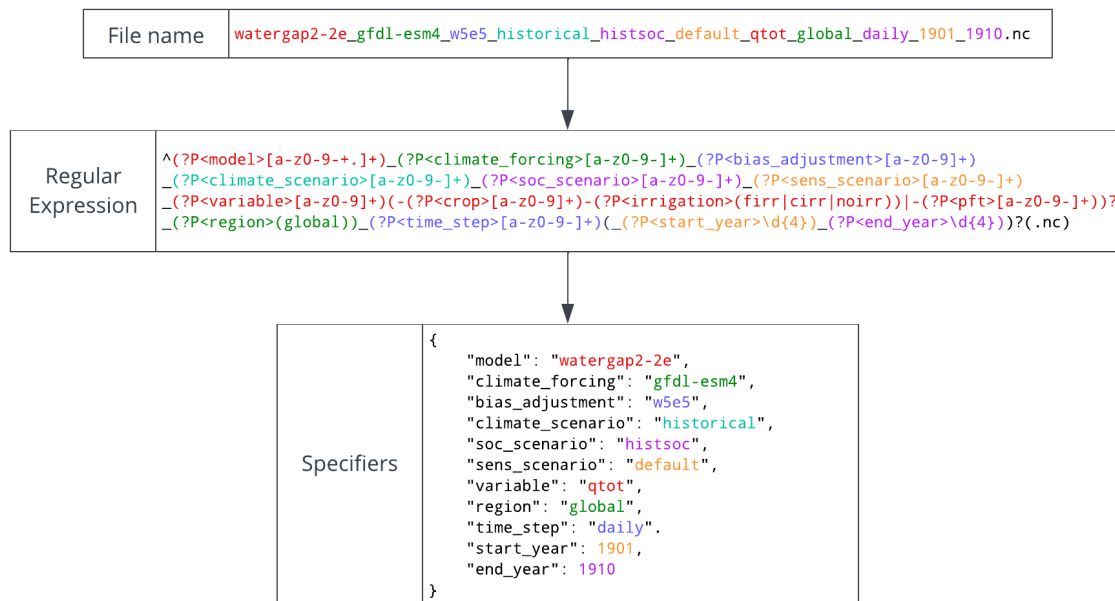
Figure 2: Metadata extraction using regular expressions: The file name consist of a set of specifiers which are defined in the ISIMIP Protocol. Using regular expressions we validate the file names and extract the specifiers into a dictionary.
