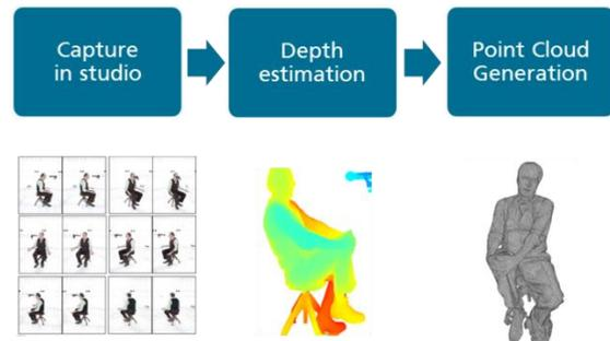
**Figure 9a:** Processing chain for volumetric video production (1)
