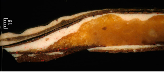
Fig. 4 Cross-section of a sample taken from the hair of Saint Erasmus head, showing four re-painting interventions
