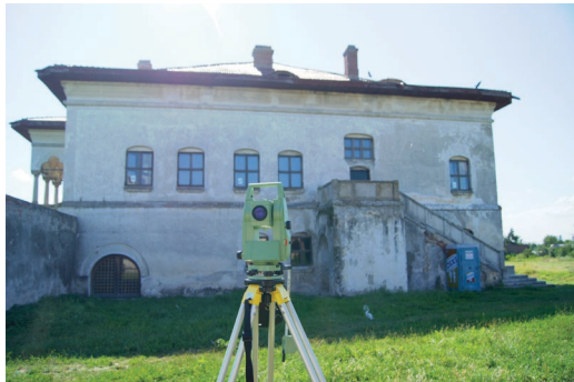
Fig. 20 Total station set up.
