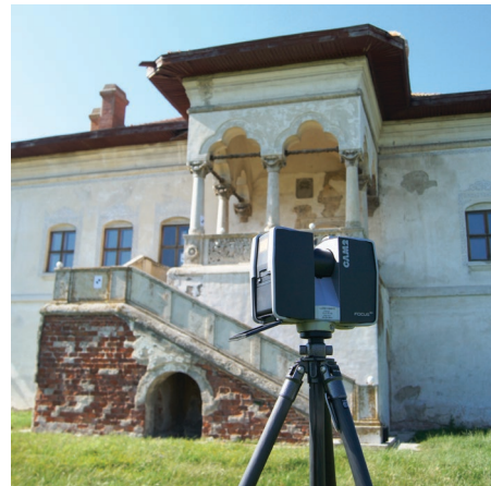
Fig. 18 3D outdoor laser scanner survey operation.
