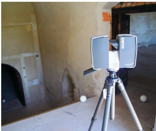
Fig. 17 3D indoor laser scanner survey operation.
