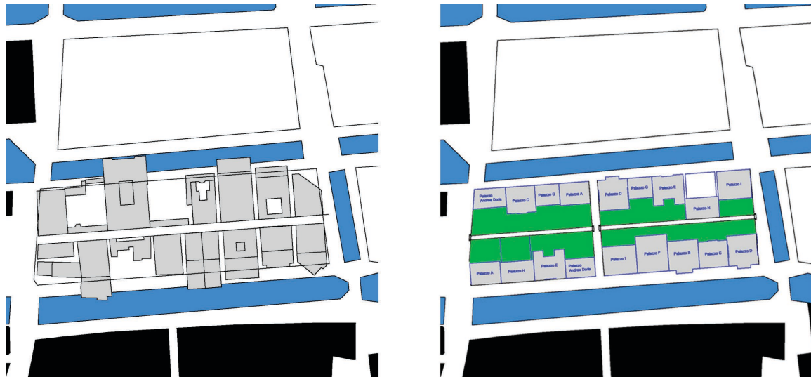
Fig. 8 Left: Projection of the Strada Nuova on the Nieuwstadt building block. Right: The proposed layout adapted, with palazzos oriented towards the canals and enclosed gardens. (Both: AutoCAD™ 2009).
