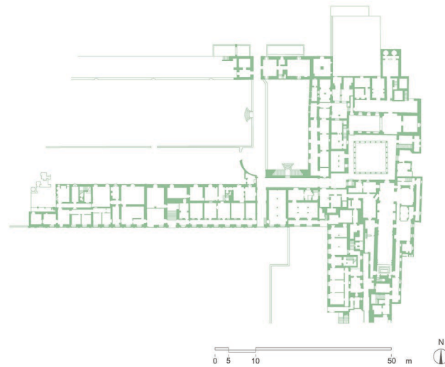
Fig. 6 Drawing of the ground floor of the Palace of Vila Viçosa, obtained by vectorization of overlapped scans of the existing plans (2012).
