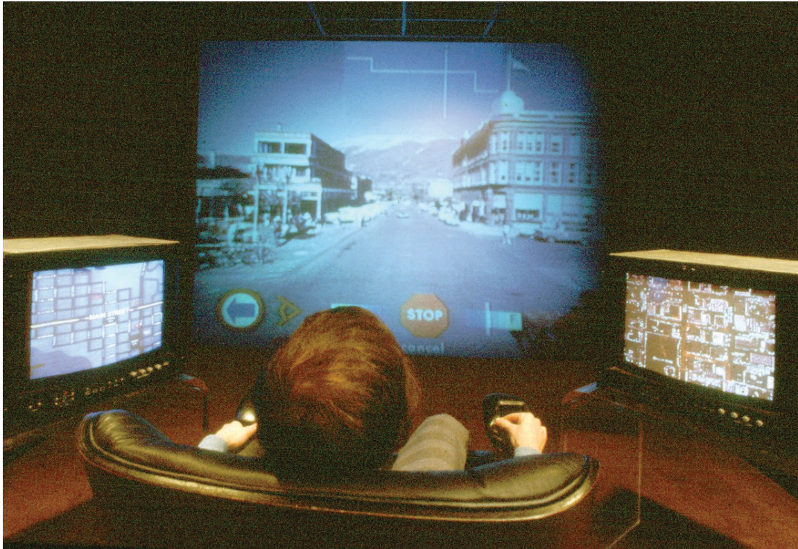
Fig. 1 The Aspen Moviemap experienced in the 'Media Room' at the Architecture Machine Group, MIT, ca 1980. The 'traveller', seated in an instrumented armchair, controls speed and direction of travel. Touch screens displaying map and aerial views allow access to additional multimedia material.
