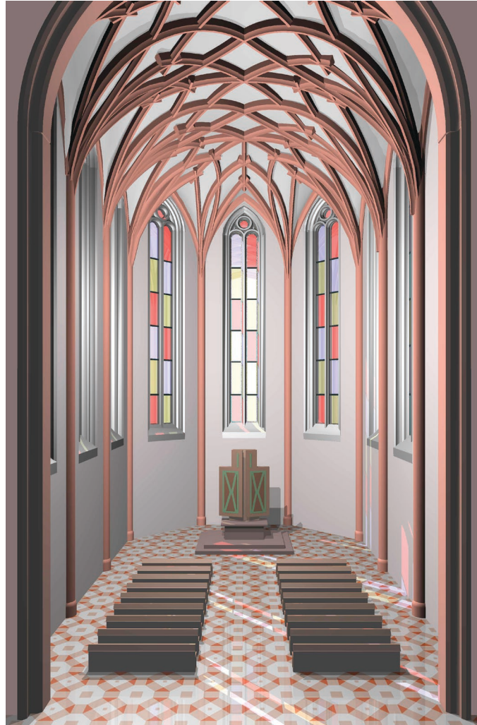
Fig. 12 Digital display of a church choir by Werner Müller and Norbert Quien (1991). The shape of the vault and the window profiles are derived from designs in the 'Stromersches Baumeisterbuch' (Nuremberg, ca 1590), which were test pieces for an examination for the master craftsmen's certificate and were not intended for actual building (compare fig. 10). The floor is modelled on a medieval example.
