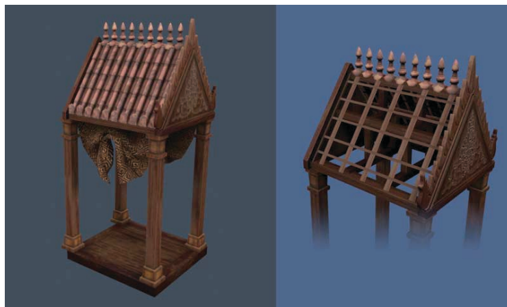
Fig. 7 3D modelling tests (2008) of wooden building components shown in the reliefs. On the left, cloth curtains hang between the pillars, and on the right, the structural framework beneath the tiles.
