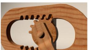
Simulating Polhem in Cinema 4D step by step – from a rudimentary three dimensional drawing to a detailed cogwheel with wooden textures.
