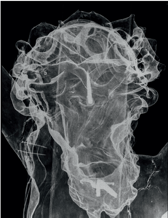
Fig. 3, 4: X-ray images of the head of Christ by Christian Ackermann which enable to detect different materials (col-our image) and to inspect the inner structure of the artefacts (black and white image) (2018).
