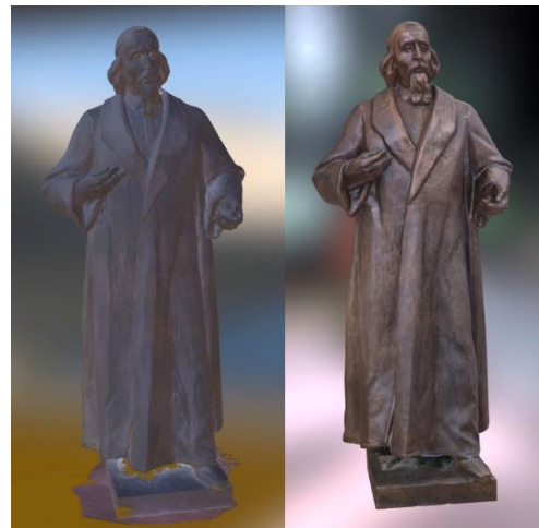
Figure 1: A 3D model of a statue of Jan Amos Komensky created using optical scanning (left) and photogrammetry (right)
