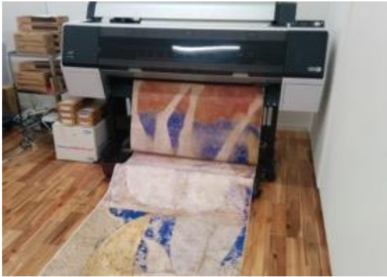
Figure 13: Printing the mural painting on Japanese washi paper as the base layer
