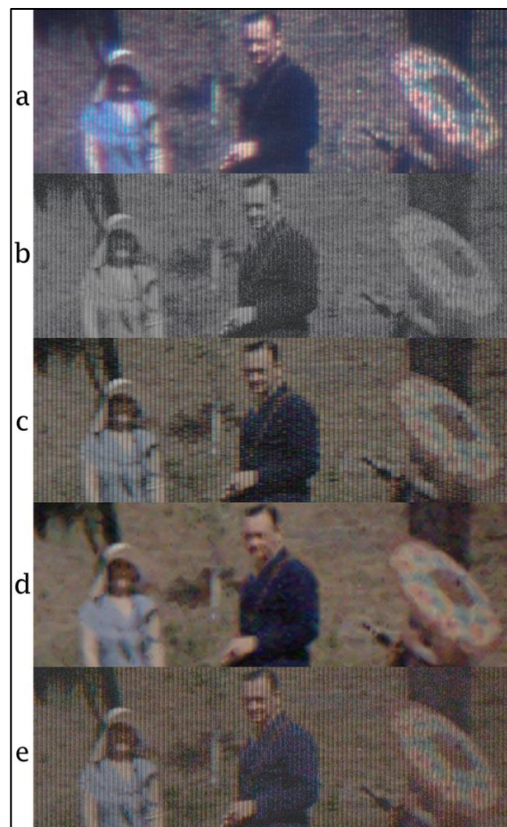
Figure 3: Frame detail of a lenticular film belonging to the collection of the Lichtspiel / Kinemathek Bern. Direct projection on color digital sensor (a), scan of silver emulsion (b) carried out by the FilmColors team. Three different color reconstructions from the scan (c, d and e) conducted by Joakim Reuteler.
