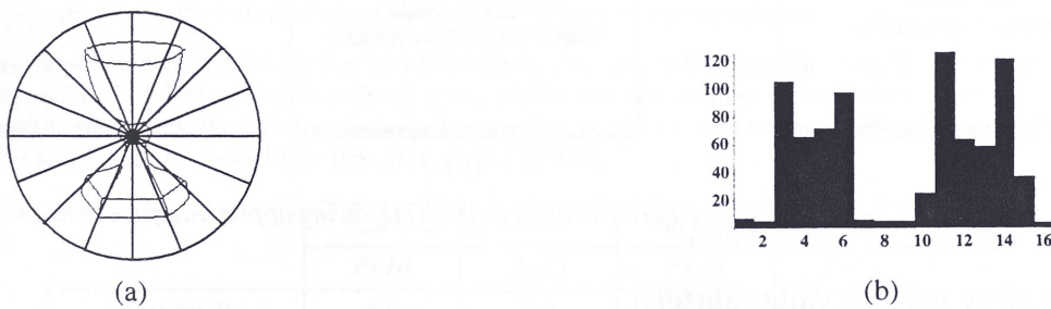
Figure 6 : Graphical representation of the circular histogram. (a) The centre of gravity of the watermark is used as the middle point to compute the circular histogram. (b) Representation of the histogram computed from the figure (a).
