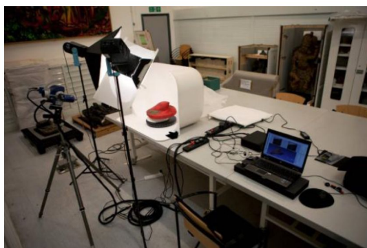
Fig.2: A typical setup for V&A scanning
