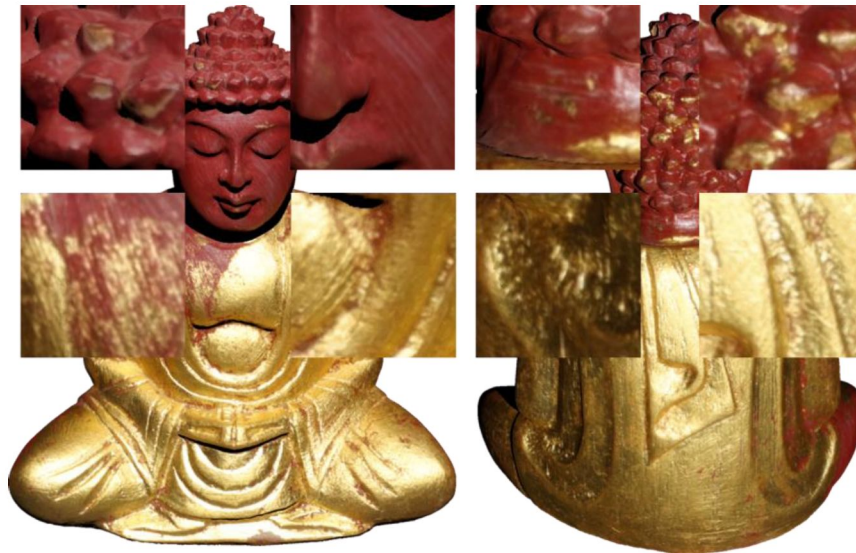
Figure 5: Achieved quality of an object acquired with the Multiview Dome object acquisition pipeline [SWRK11], employing a 3D reconstruction obtained with structured light [WSRK11] together with BTF reflectance data.
