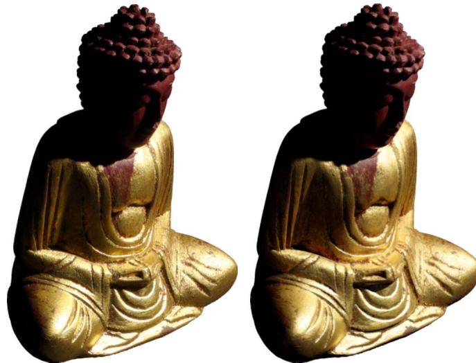
Figure 6: Test of faithfulness of the Multiview Dome acquisition. Left: Picture taken with calibrated camera and light-source. Right: Rendering of digitized object under the same view and light conditions.
