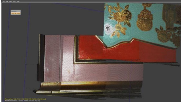
Figure 6: Highlights and brightness non-uniformity visible on separate scans
