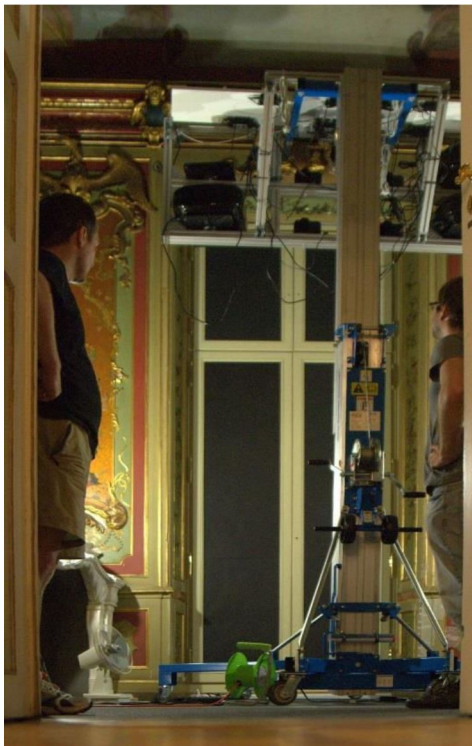
Figure 3: Measurement system mounted on the positioning device
