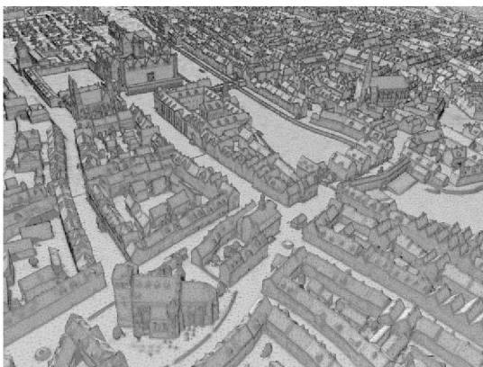
Figure 12: The triangulated surface data of the Berlin city model 3D scan
