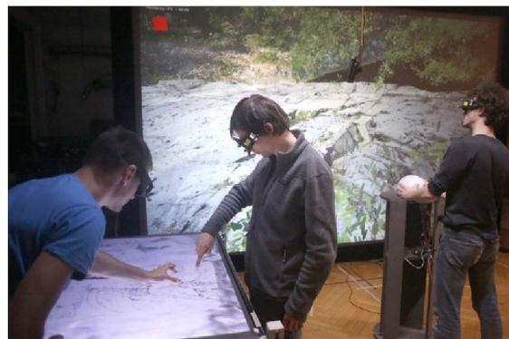
**Figure 7:** Early tests with the implementation of the 3D-Pitoti Scientists lab at Bauhaus-Universität Weimar. The real-time point-cloud rendering system has been integrated in the multi-user capable 3D rendering and interaction system Guacamole [5]. Here, two users inspect the detailed structures of a rock-art figure, while another one, explores the surrounding.
