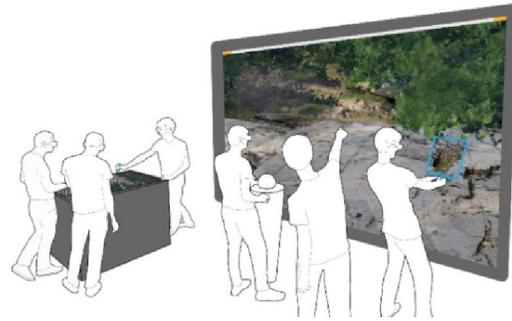
**Figure 6:** Illustration of the 3D-Pitoti Scientists Lab. A large 3D screen affords the exploration of the 3D scanned environment from an egocentric perspective, while the 3D tabletop better supports a bird's-eye viewpoint. Both displays can be used effectively for the analysis of geometric details. The system supports virtual "photos" for the individual capturing and preparation of interesting perspectives and content transfer between physical display devices.
