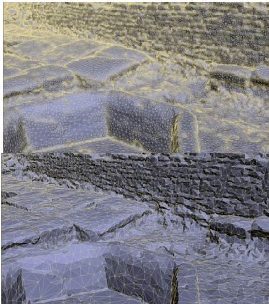
Figure 6: The polygon-reduction of a 3D model significantly diminishes its quality, as shown by a detail view on the front part of the Roman temple of Neuenstadt am Kocher. Top: high-resolution model; bottom: low-resolution model. Note how details like the bricks of the wall in the background become blurred in the low-resolution model.
