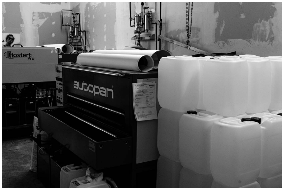
9] Kenneth C. Korfmann, developing machine Contimat SW 130-200 from Autopan for color photography, Tricolor Photoprint GmbH, Adliswil, February 28, 2024, 1:06 p.m., Leica SL2, 43 mm, f/14, 1/20 s, ISO 800.
